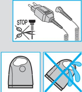
To prevent the cleaning fluid from leaking, ensure that the Clean&Renew station is placed on a flat surface. When a cleaning cartridge is installed, do not tip, move suddenly or transport the station in any way as cleaning fluid might spill out of the cartridge. Do not place the station inside a mirror cabinet, nor place it on a polished or lacquered surface.
