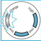
The red low charge segment flashes when the battery capacity has dropped below 20%, provided the shaver is switched on. The remaining capacity will then be sufficient for 2 to 3 shaves.
